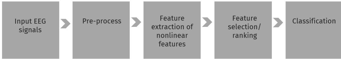
Figure 2: A typical block diagram of a CAD system.
